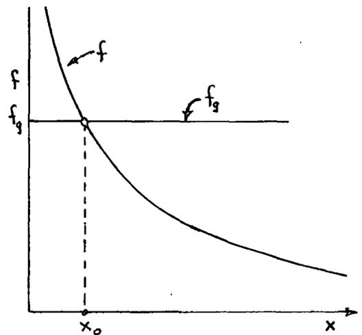
A solution to this equation is shown graphically in the figure. The equilibrium is statically unstable because if the mass moves in the positive x direction from  $x_0$ , the gravitational force exceeds the magnetic force and tends to carry it further from equilibrium.
