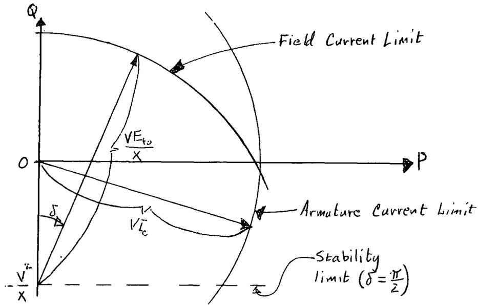
The stability limit ( $\delta = \frac{\pi}{2}$ ) is also shown in the sketch, along with the armature current limit.
