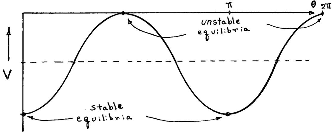
Here it is clear that there are points of zero slope (and hence zero torque and possible static equilibrium) at
