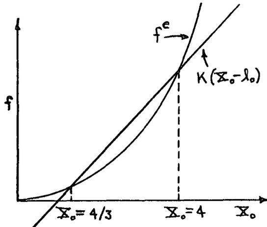
Consider the equilibrium at  $x_0 = 4$ . A small displacement to the right makes the force  $f^e$  dominate the spring force, and this tends to carry the mass further in the  $x$  direction. Hence, this point is unstable. Similar arguments show that the other point is stable.
