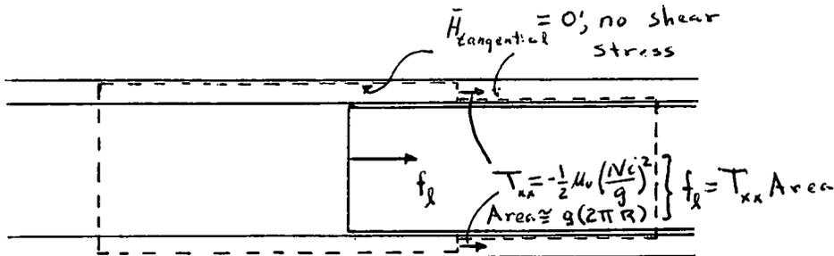
and the mirror-image is acceptable for the right-hand transducer. Application of  $f_x = \oint_S T_{xj} n_j da$  to the two surfaces yields the same result as in part (a).
