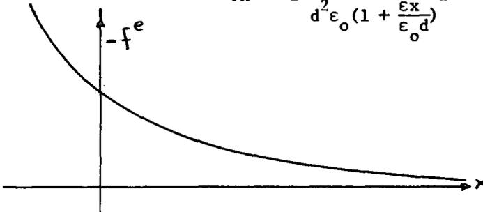
The energy converted to mechanical form is  $\int f^e dx$ . The contribution to this integral from  $d \rightarrow c$  and  $b \rightarrow a$  in the figure is zero. Hence,
