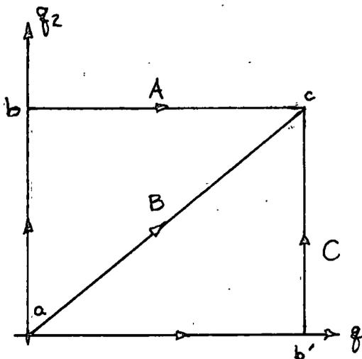
First carry out this line integral along the contour A: from  $a \rightarrow b$ ,  $q_1 = 0$ , while from  $b \rightarrow c$ ,  $dq_2 = 0$ . Hence,
