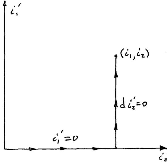
Sec. 3.1.1). The co-energy input through the electrical terminal pairs with the mechanical system held fixed is
