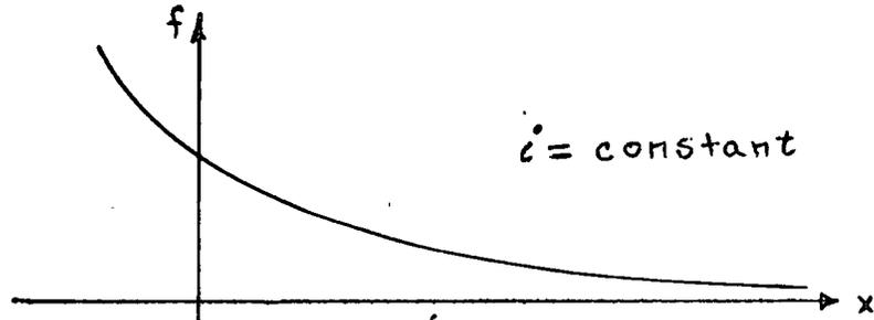
With the current constant, the drop in  $\int \vec{H} \cdot d\vec{l}$  across the gap increases with  $x$ , and hence the field in the gap is reduced by increasing  $x$ .
