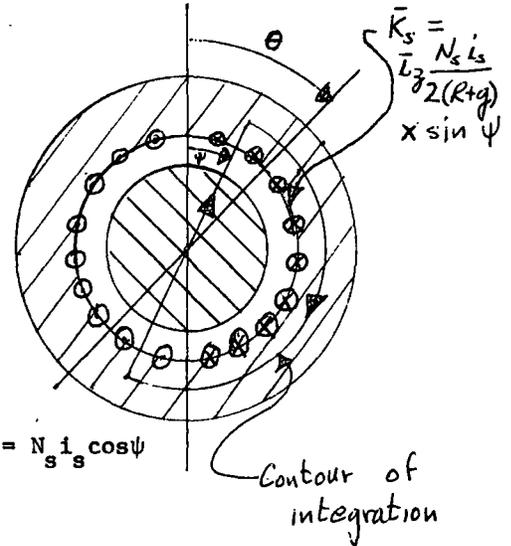
$$2H_{rs}(\psi)g = \int_{\psi}^{\psi+\pi} \left[ \frac{N_s i_s}{2(R+g)} \sin \psi' \right] (R+g) d\psi' = N_s i_s \cos \psi$$
