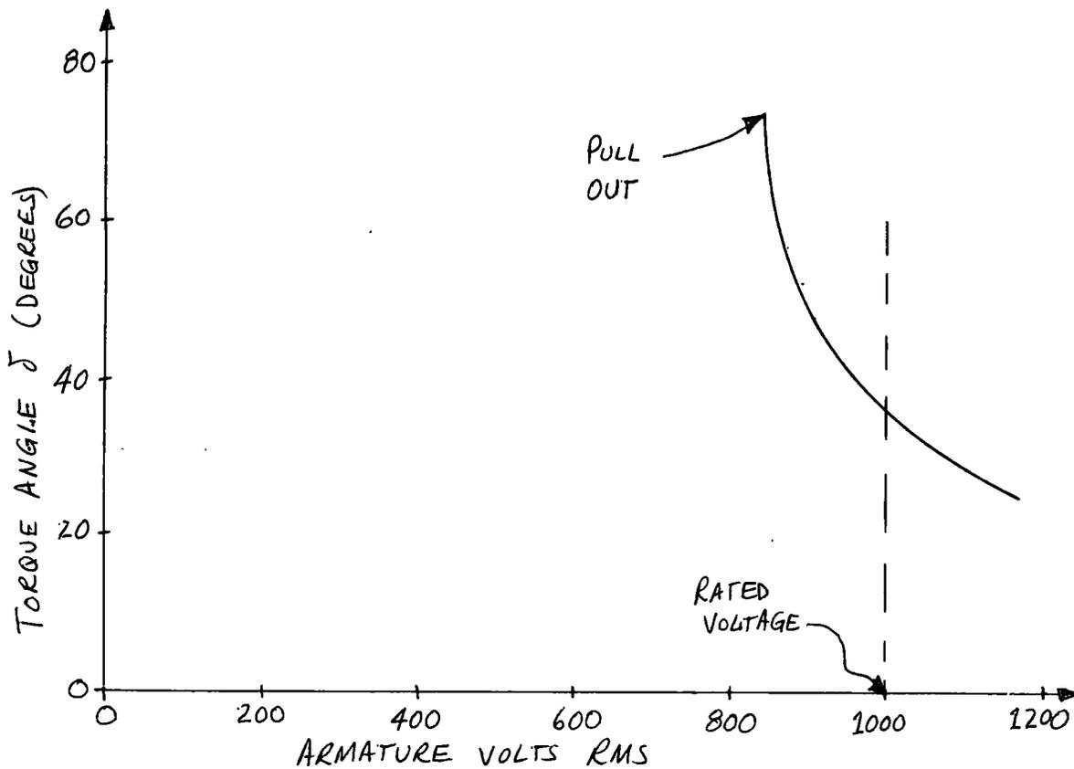
Although it was not required for this problem, calculations will show that operation at reduced voltage will lead to excessive armature current, thus, operation in this range must be limited to transient conditions.
