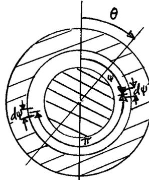
$$d\lambda_s = \underbrace{\left[ \frac{N_s}{2(R+g)} \sin\psi \right]}_{\text{number of turns in elemental coil}} (R+g) d\psi \underbrace{\left[ \int_{\psi}^{\psi+\pi} B_r(\psi') (R+g) \ell d\psi' \right]}_{\text{flux linking one turn of elemental coil}}$$
