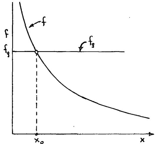
A solution to this equation is shown graphically in the figure. The equilibrium is statically unstable because if the mass moves in the positive x direction from  $x_0$ , the gravitational force exceeds the magnetic force and tends to carry it further from equilibrium.
