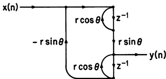
Coupled form implementation of a complex conjugate pole pair. (Note that the transfer function has been corrected. The numerator factor is  $r \sin \theta$  not  $r \cos \theta$  as indicated in the lecture.)
