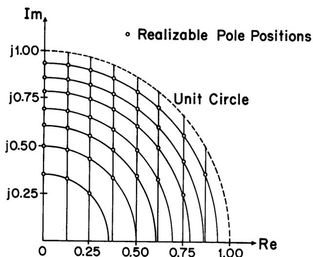
Grid of possible pole locations for the network of viewgraph  $f$  when the coefficients are quantized to three bits.
