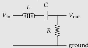
$$G(\omega) = \frac{\frac{j\omega}{\omega_0}}{1 + \frac{j}{Q} \frac{\omega}{\omega_0} - \frac{\omega^2}{\omega_0^2}} \quad (3.107)$$
