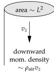
$$mg \sim \rho_{\text{air}} v_z^2 L^2, \quad (3.91)$$
