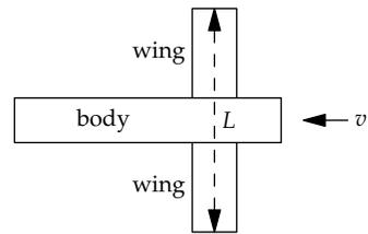
$$F_{\text{drag}} = \rho_{\text{air}} v^2 \times \begin{cases} CL^2 \\ \frac{1}{2} c_d A_{\text{cs}} \end{cases} \quad (4.69)$$
