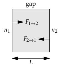
$$\begin{aligned} F_{1 \rightarrow 2} &\sim n_1 \frac{D}{L} \\ F_{2 \rightarrow 1} &\sim n_2 \frac{D}{L}. \end{aligned} \quad (7.54)$$
