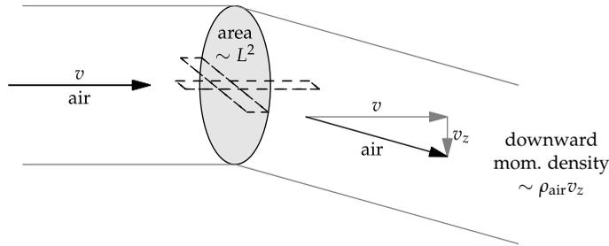
Before the air reaches the wing (the left tube), the air has zero downward momentum. As in the analysis of hovering flight, the Earth supplies downward momentum to the plane, which passes it onto the air. This downward momentum is carried away by the air after the wing (the right tube).
