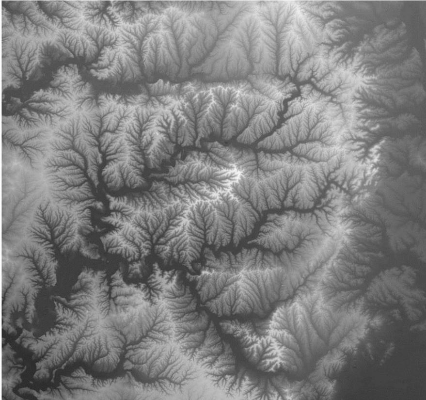
Digital Elevation Model (DEM): A sampled array of elevations for a number of ground positions at regularly spaced intervals
